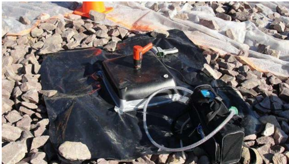
Photograph 9-15 View of a bus tub with shroud
