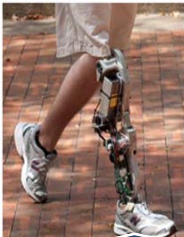
NIH supported researchers are developing a powered robotic prosthesis that senses a person's next move and provides powered assistance to achieve a more natural gait.
