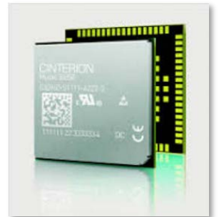
Figure 1. Thales Cinterion EHS8 module used in millions of IoT devices.
